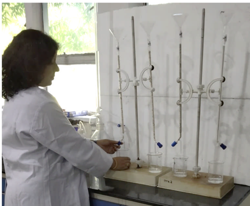
Figure 6.1: Photograph of the lab-scale AMD remediation process
